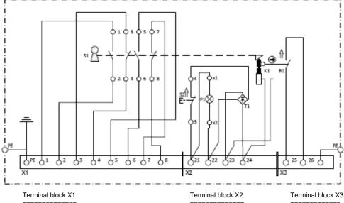
Rated operating voltage: max. 500 V Rated operating current: max. 20 A Rated surge voltage: max. 6 kV
